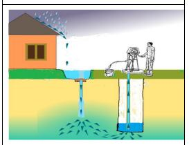
Photo 4. A drawing of the Tube recharge. Water from a roof and/ or ground collects in the pit
