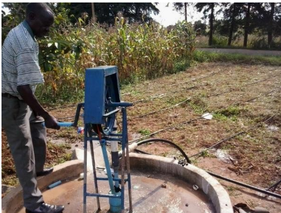
Low pressure drip irrigation. The hoses need a head of 70cm and can be directly mounted to the outlet of a Rope pump.
