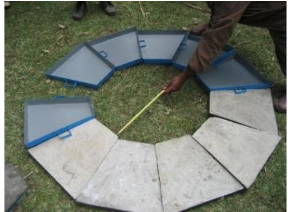
Fabrication of well-reducer rings which allow the installation of pumps on wells with a large diameter
