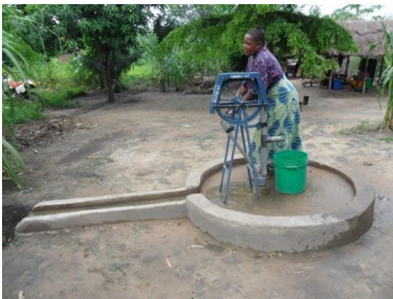
Rope pump – Model 1. A hand pump that is locally produced by trained companies. The cost ranges between $70 and $130/pump, depending on the model. The Rope pump can pump from up to 35m of depth and is easy to maintain.
