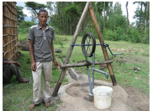
Rope pump – Pole model. The Pole model is often used for irrigation and can be mounted on any size of well.
