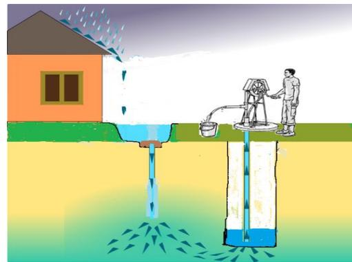
Photo 4. A drawing of the Tube recharge. Water from a roof and/ or ground collects in the pit
