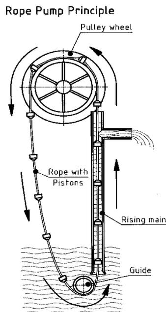
**Photograph 1. Schematic drawing of a Rope pump**
